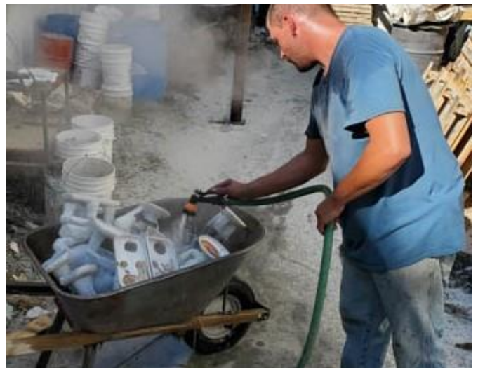
Newly Bronze-filled Plaster Molds Being Cooled
