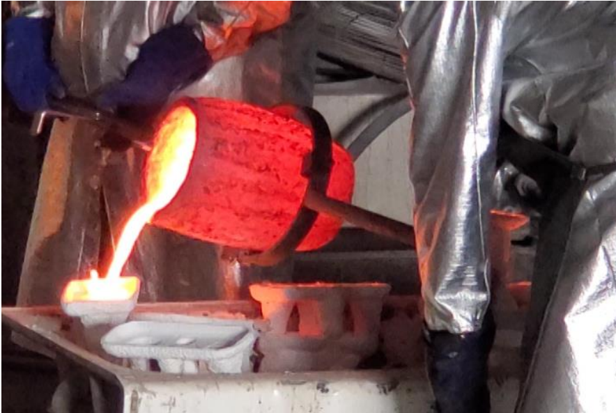
Molten Metal Being Poured into Molds
